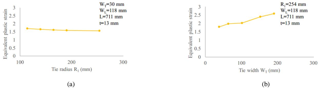
Figure 11. Equivalent plastic strain with: (a) Variations in  $R_1$ , (b) Variations in  $W_T$
