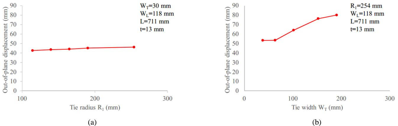
Figure 10. Out-of-plane displacement with: (a) Variations in  $R_1$ , (b) Variations in  $W_T$
