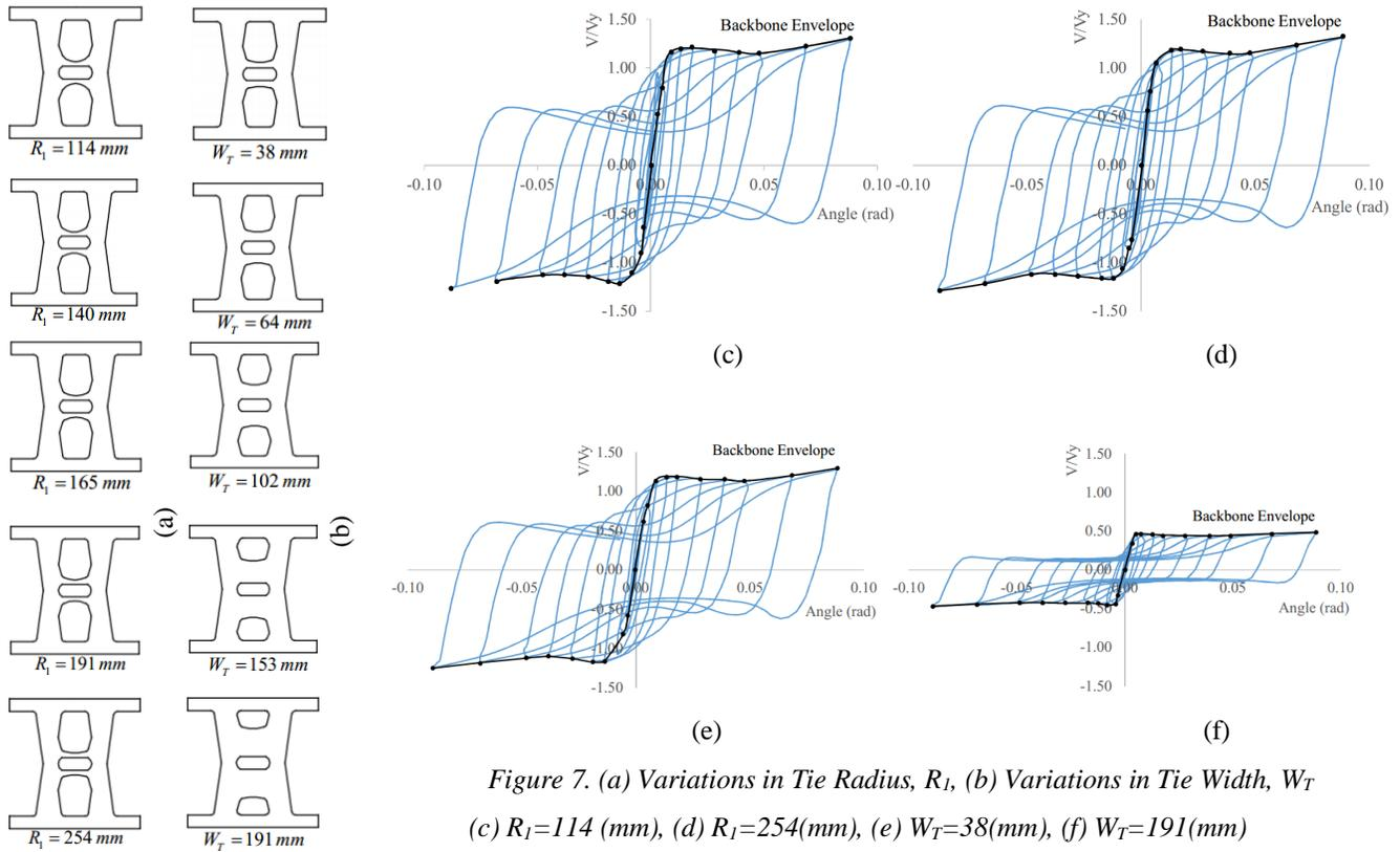
Figure 7. (a) Variations in Tie Radius,  $R_I$ , (b) Variations in Tie Width,  $W_T$  (c)  $R_I=114$  (mm), (d)  $R_I=254$ (mm), (e)  $W_T=38$ (mm), (f)  $W_T=191$ (mm)
