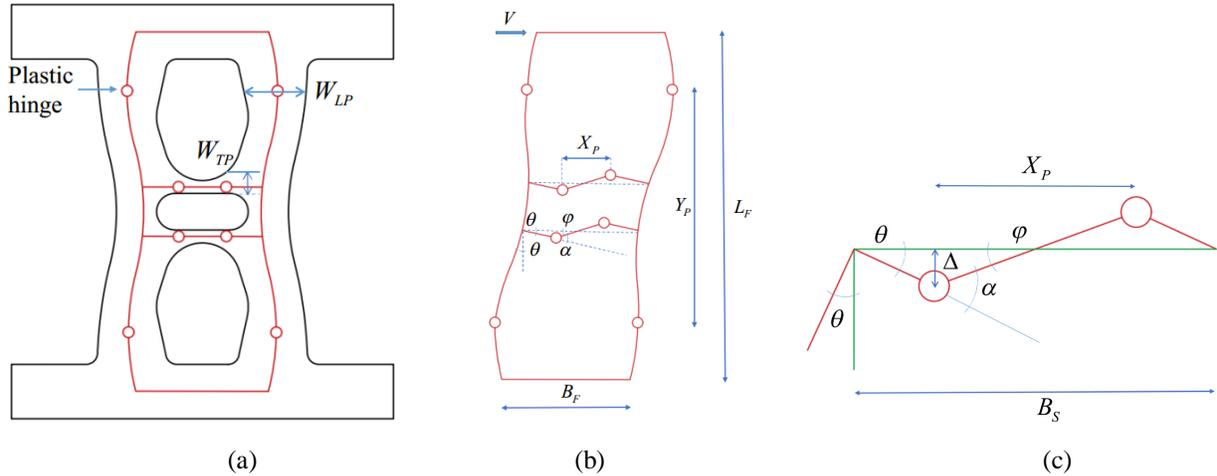
Figure 5. (a) Un-deformed shape, (b) Deformed shape, (c) Tie configuration
