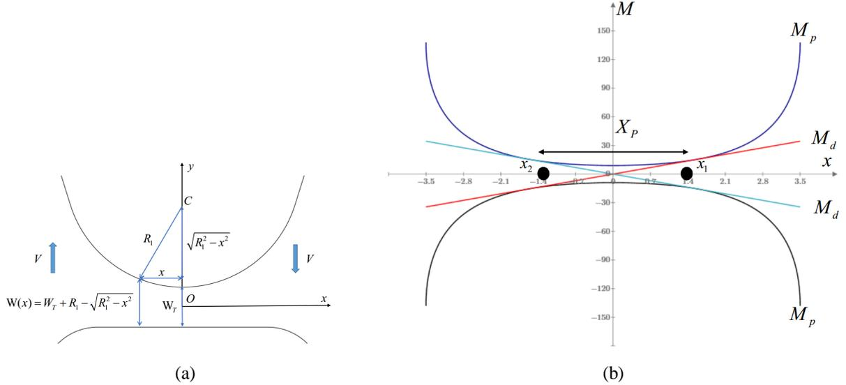
Figure 6. (a) Local coordinate system, (b) Locations of plastic hinges
