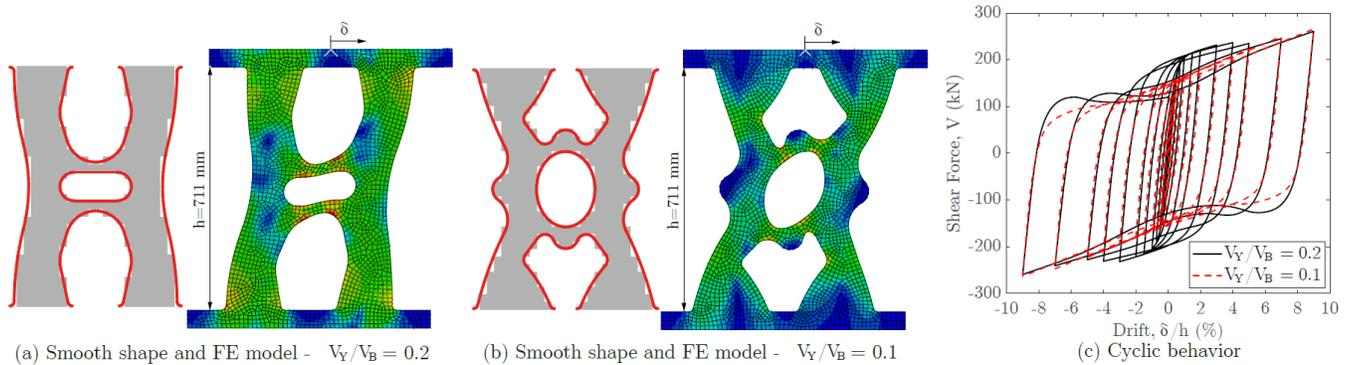
Figure 3: Cyclic behavior of both optimized topologies
