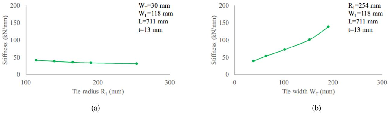
Figure 9. Stiffness with (a) Variations in  $R_1$ , (b) Variations in  $W_T$
