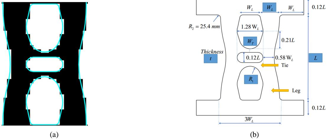
Figure 4. (a) Smoothed curves over pixelated topology, (b) Parameters
