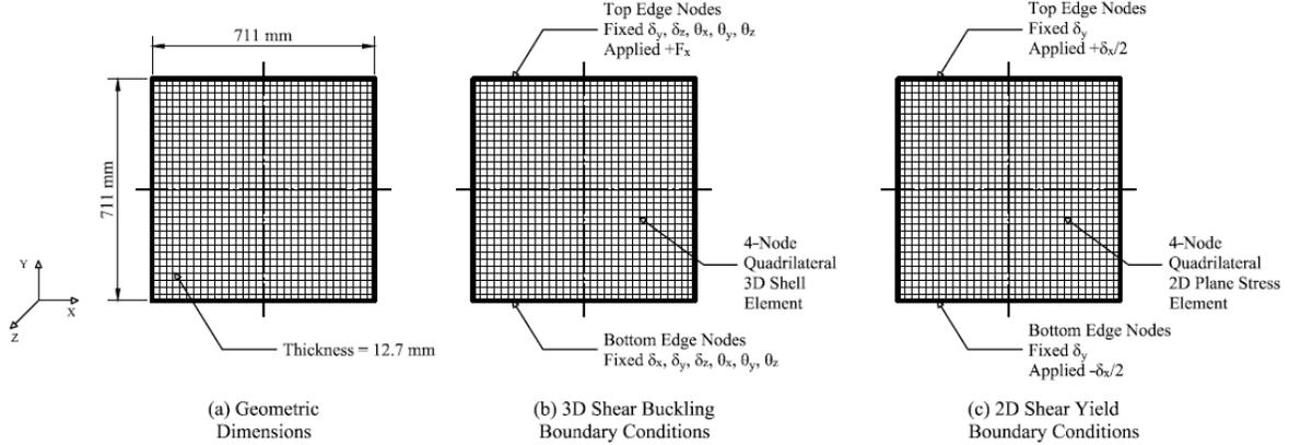
Figure 1. Domain and boundary conditions for finite element analyses
