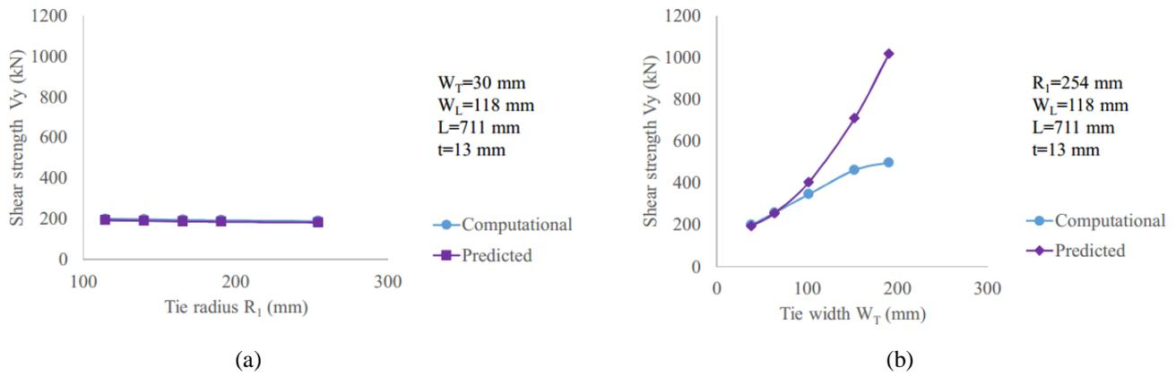
Figure 8. Strength with (a) Variations in  $R_1$ , (b) Variations in  $W_T$
