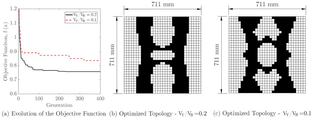
Figure 2: Evolution of the objective function and optimized topologies for a target volume of 40%
